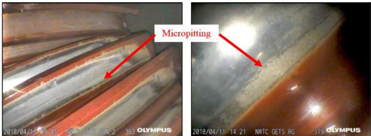
Figure 4 – Micropitting on the sun pinion teeth. (Photos by Scott Eatherton, Wind Driven, NREL 61193 and 61194)
