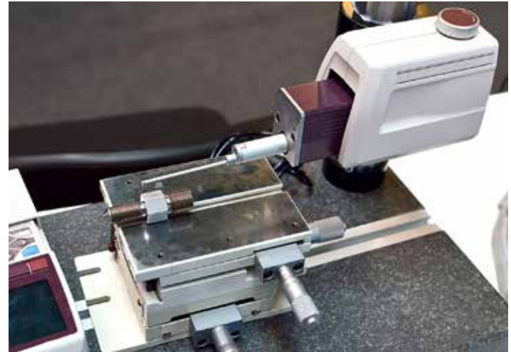
A profilometer used for measuring surface texture. (Courtesy: Shutterstock)
