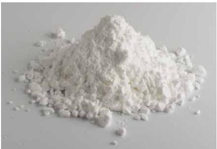
The abrasive, typically aluminum oxide, can vary in grit size. The ceramic binder starts out as clay. Media manufacturers will blend abrasive and clay together in different ratios and use abrasives of different grit sizes to generate a myriad of compositions.
