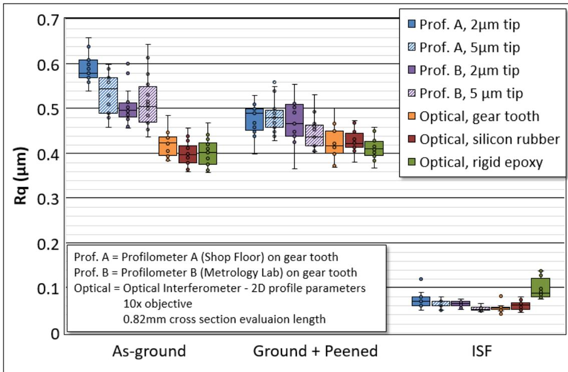
Figure 8 - Rq, profilometer vs. interferometer results
