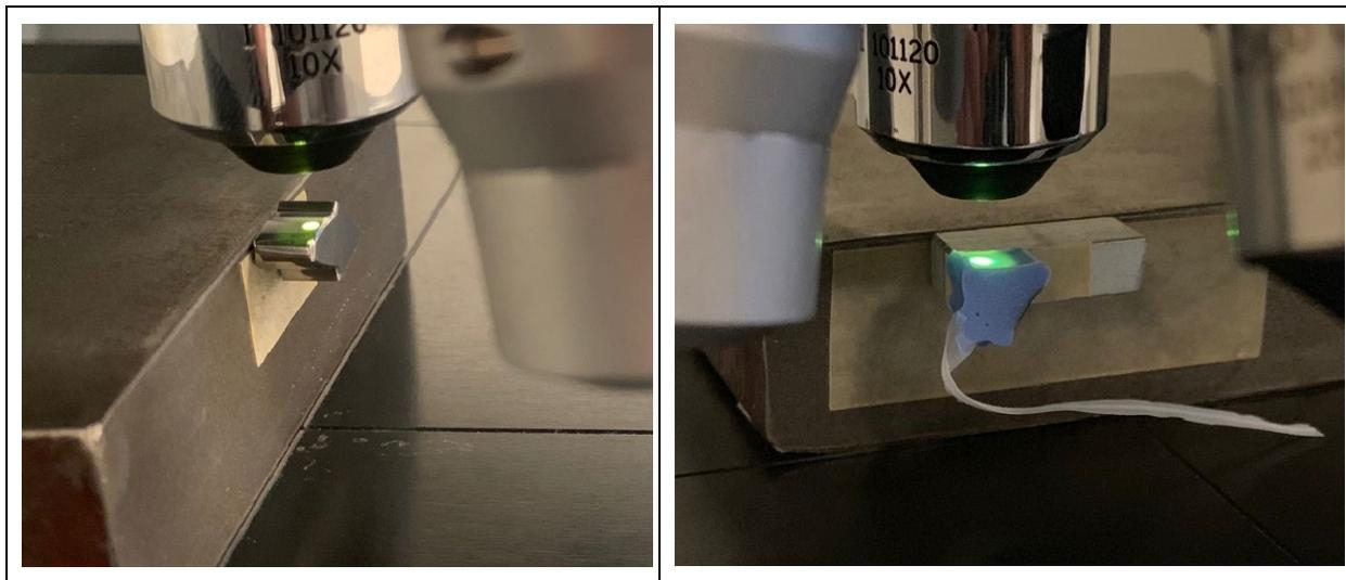
**Figure 5 - Gear tooth and hard epoxy replica in interferometer**
