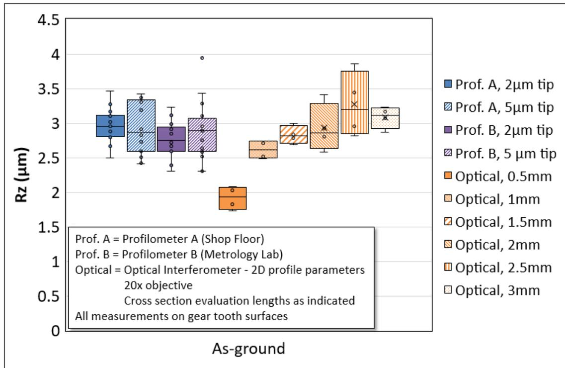
Figure 16 - Effect of scan length on Rz
