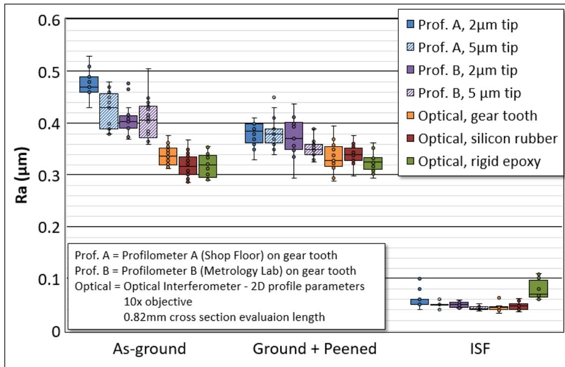
Figure 7 - Ra, profilometer vs. interferometer results
