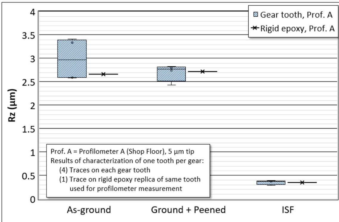
Figure 20 - Rz comparison, rigid epoxy vs. gear teeth
