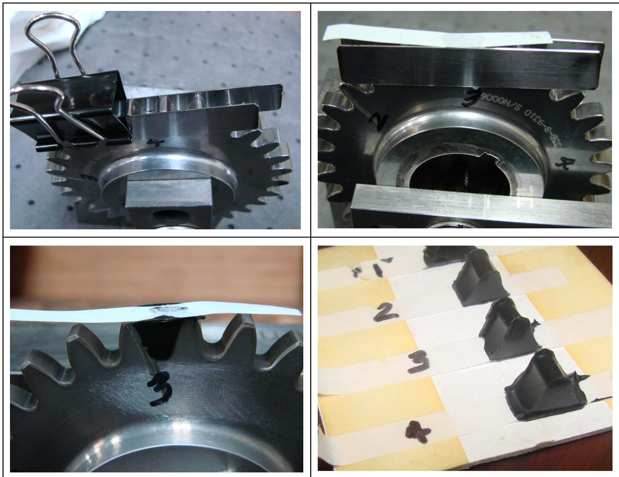
**Figure 1 - Silicon rubber replication process**
