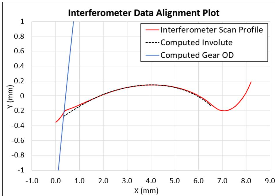
**Figure 12 - Aligning scan data of a tooth replica to a mathematically generated involute**
