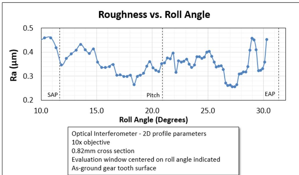
**Figure 13 - Roughness vs. roll angle of an as-ground gear tooth surface**
