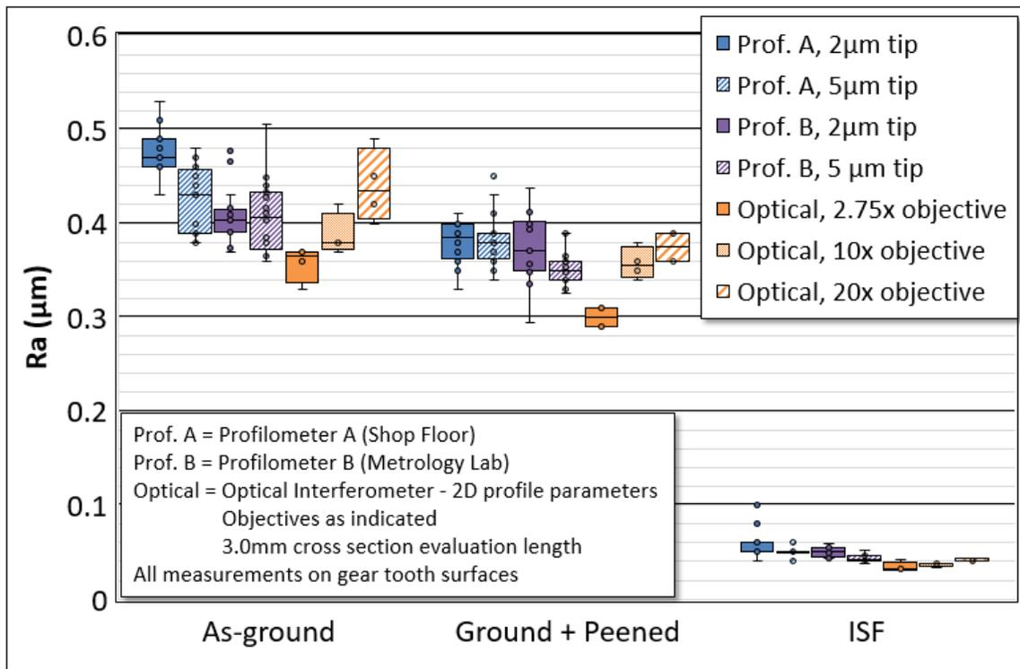
Figure 17 - Objective lens selection effect on  $R_a$
