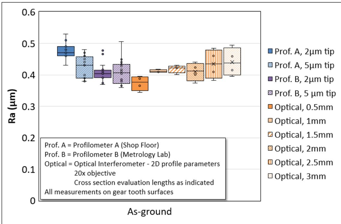
Figure 15 - Effect of scan length on Ra
