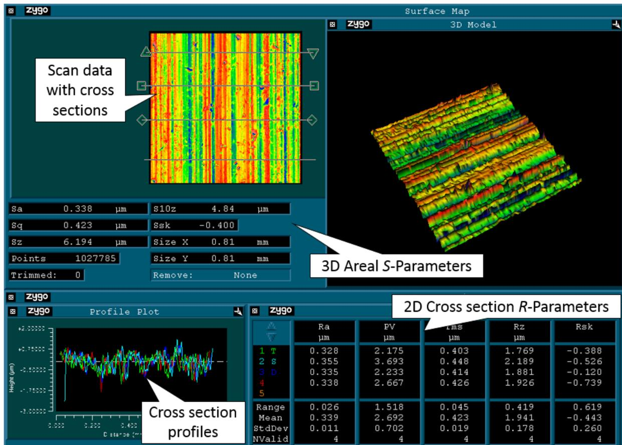
**Figure 6 - Processing of interferometry data**
