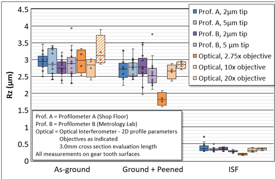
Figure 18 - Objective lens selection effect on  $R_z$
