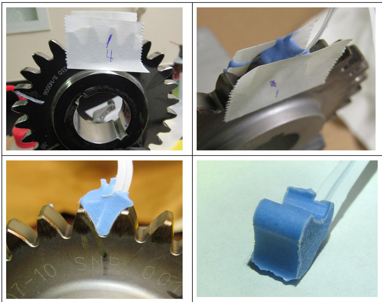
Figure 2 - Hard epoxy replication process
