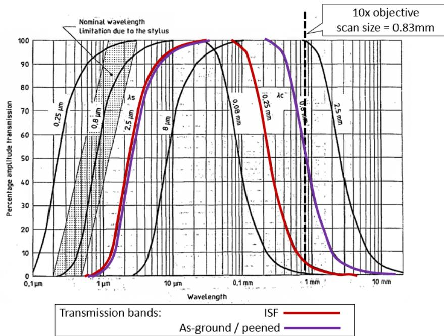
Figure 14 - Gaussian filter transmission characteristics (from ISO 3274, with markups)
