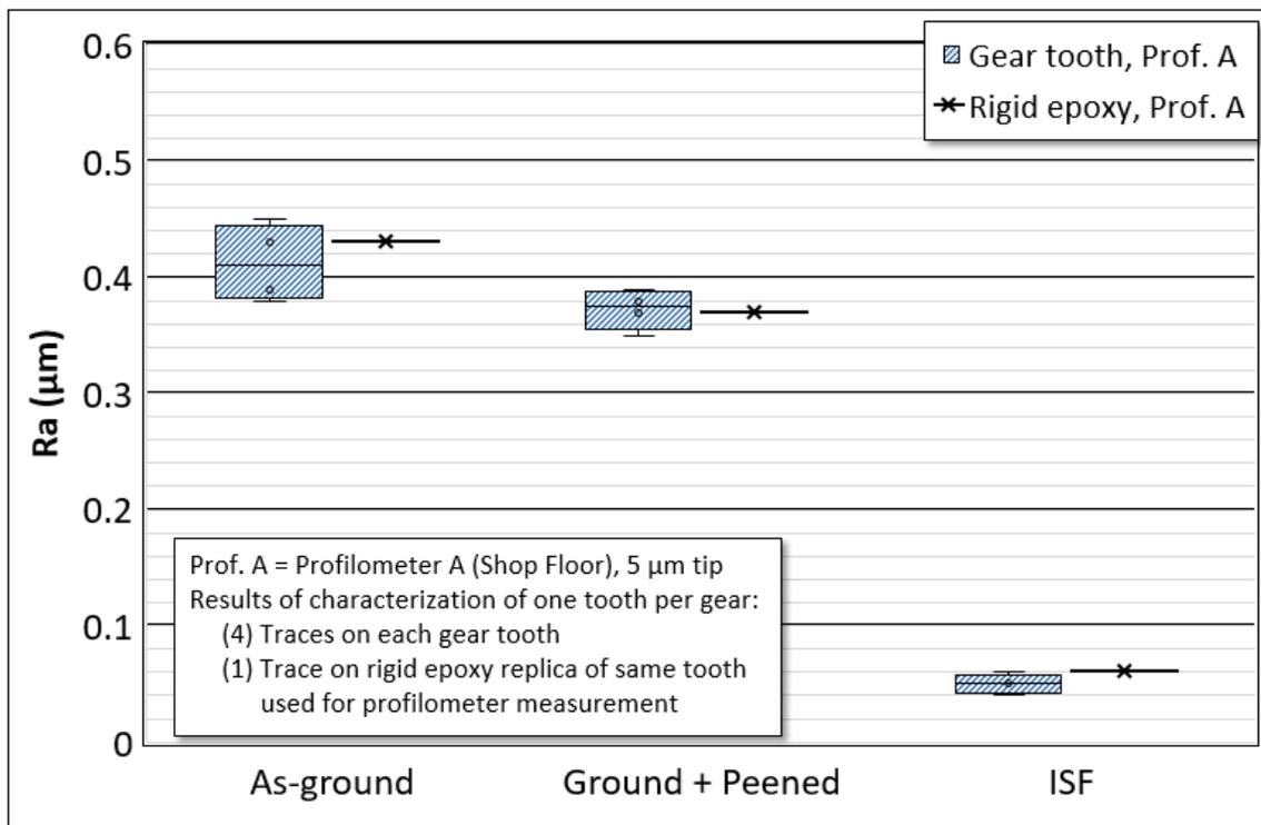
Figure 19 - Ra comparison, rigid epoxy vs. gear teeth
