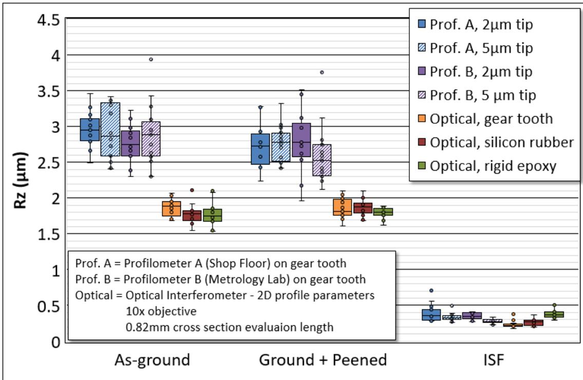
Figure 9 - Rz, profilometer vs. interferometer results
