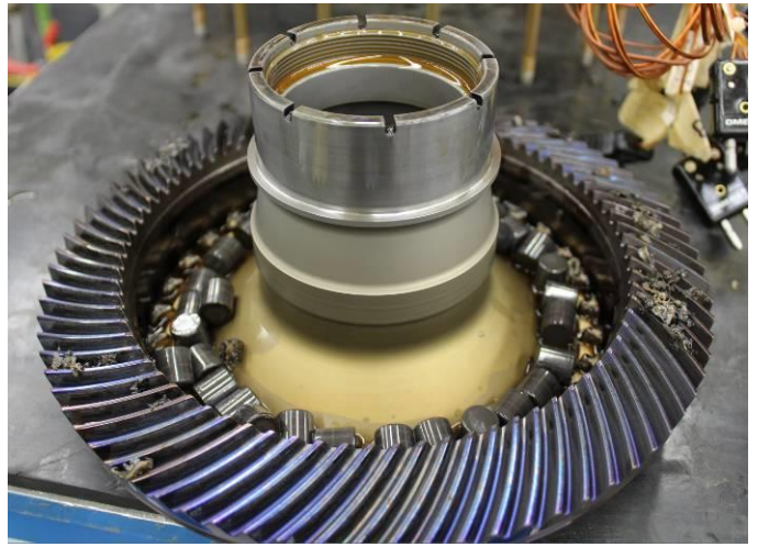
Figure 11. FARDS MRGB LOL with PEEK bearing cages – gearshaft.
