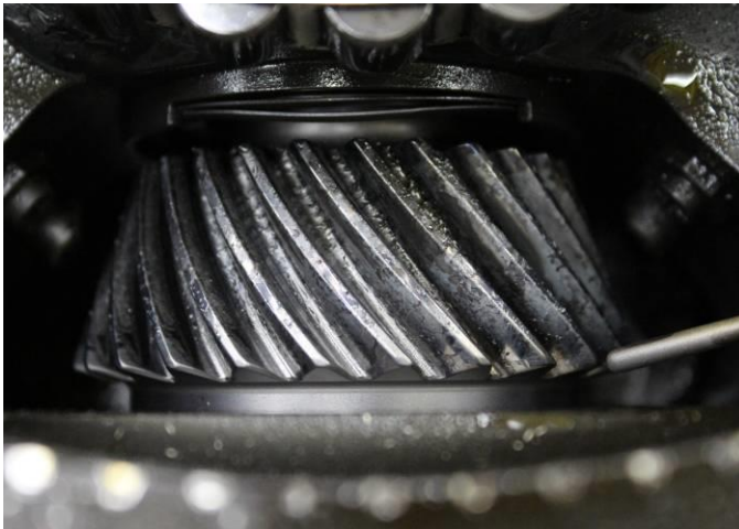
Figure 22. FARDS MRGB LOL without heat pipes and steel bearing cages – input pinion.
