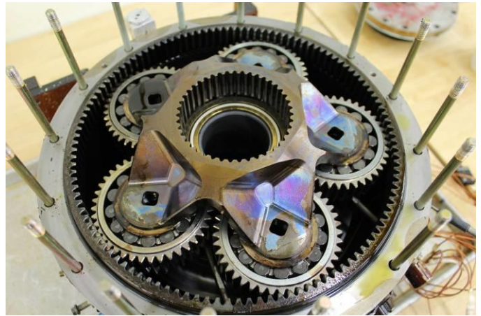
Figure 18. FARDS MRGB LOL without heat pipes and steel bearing cages – top case removed.
