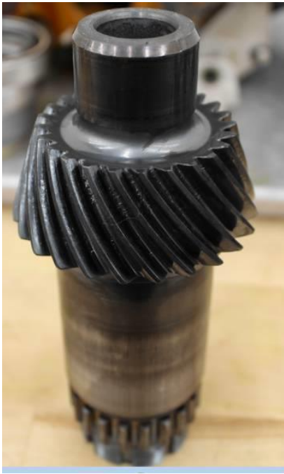
Figure 17. FARDS MRGB LOL with steel bearing cages – input pinion.
