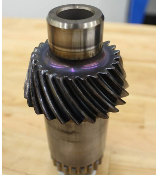
Figure 12. FARDS MRGB LOL with PEEK bearing cages – input pinion.
