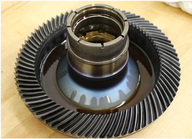
Figure 21. FARDS MRGB LOL without heat pipes and steel bearing cages – gearshaft.
