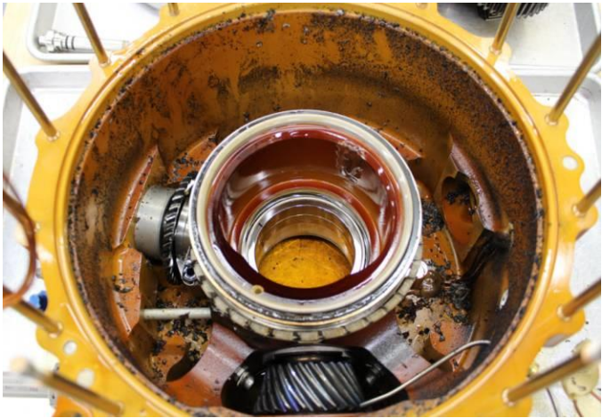
Figure 10. FARDS MRGB LOL with PEEK bearing cages – bottom of case.
