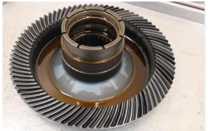
Figure 16. FARDS MRGB LOL with steel bearing cages – gearshaft.
