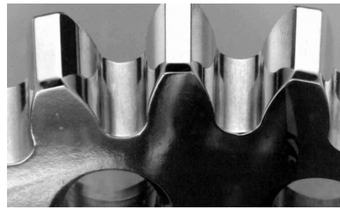
Fig. 8 Gear displaying root fillet finishing
