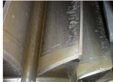
Fig. 16 Example of Scuffing on a Wind Turbine Intermediate Pinion
