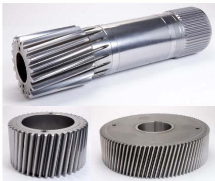
Fig. 26 Post ISF wind turbine gears (top) sun pinion, (bottom left) planet, (bottom right) low speed helical gear
