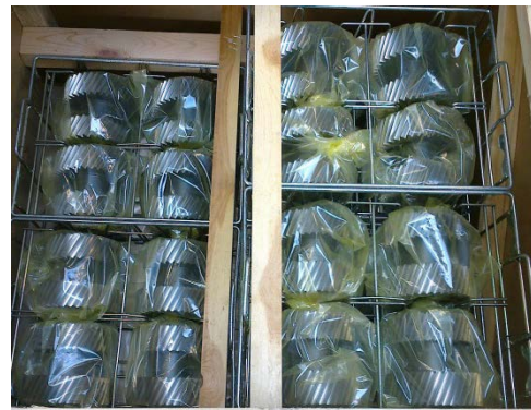
Fig. 33 Aerospace double helical gears
