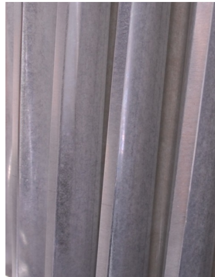
Fig. 45 Close-up of used, full isotropic superfinish planet gear
