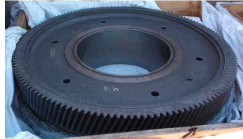
Fig. 36 Clipper Liberty gearbox double helical bull gear; approximate weight of 10,000 lbs. (~4,550 kgs.)
