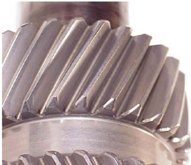
Fig. 21 Boeing CH-46 Input Pinion post ISF (Ref. 9)
