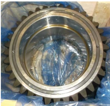
Fig. 31 Wind turbine planet gear with integral bearing race
