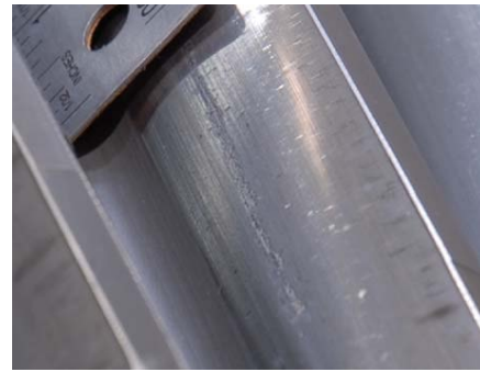
Fig. 15 Example of Micropitting on a Wind Turbine Sun Pinion
