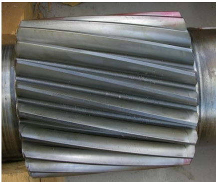
Fig. 39 Used, ground intermediate pinion
