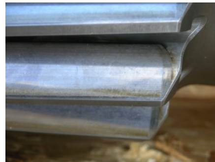
Fig. 41 Close-up of used, partial isotropic superfinish sun pinion – defined edge contact pattern
