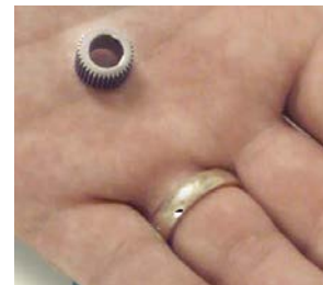
Fig. 37 Spur gear with diametral pitch of 64
