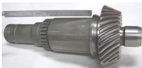
Fig. 27 Bell 427 input pinion post ISF
