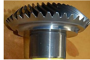
Fig. 32 Helicopter pinion with bearing surface
