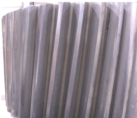
Fig. 44 Used, full isotropic superfinish planet gear
