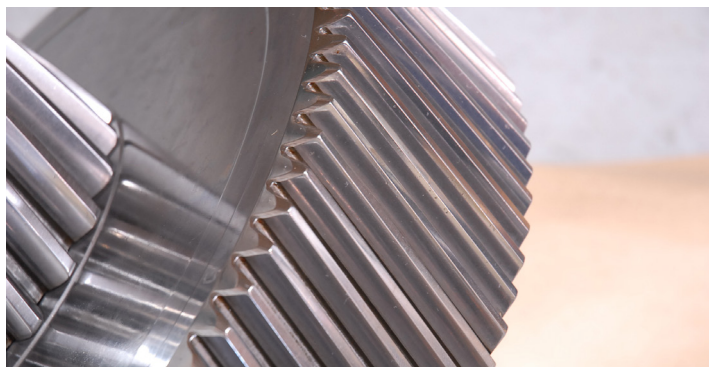
Figure 1: Used intermediate assembly after isotropic superfinishing
