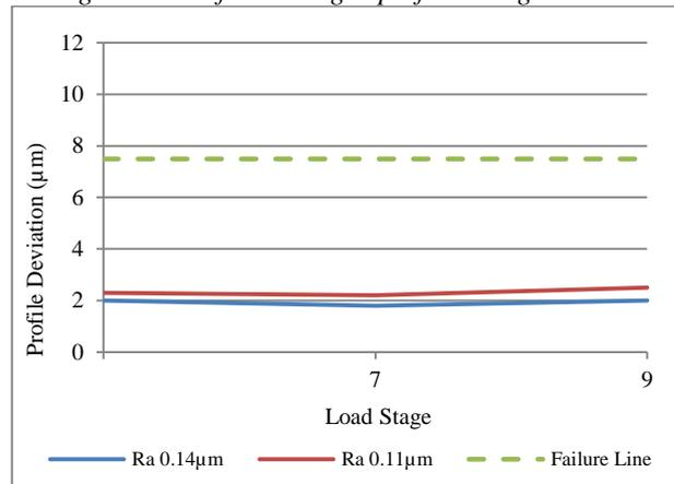
To summarise the results the average profile deviation is shown in Table 3. This result indicates that isotropic superfinished gears are resilient to micropitting with minimal profile deviation documented. This is in contrast to the ground gears that showed a 16 fold increase in profile deviation compared to the superfinished gears.
