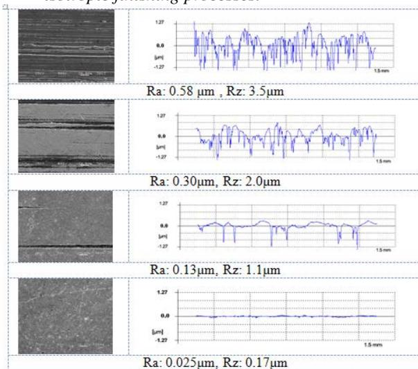
Chemically accelerated vibratory finishing is one such subset of isotropic superfinishing. This technique is applicable to a range of metallic parts such as gears and bearings and is able to reduce the Ra < 0.1µm and
