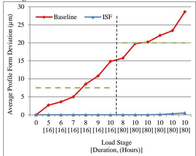
Table 5. Test 2 results after load and endurance test.
