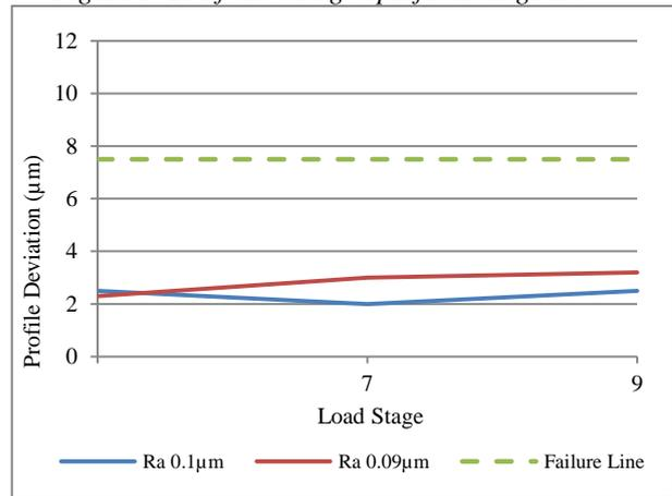
Figure 4. Brief test using superfinished gears.
