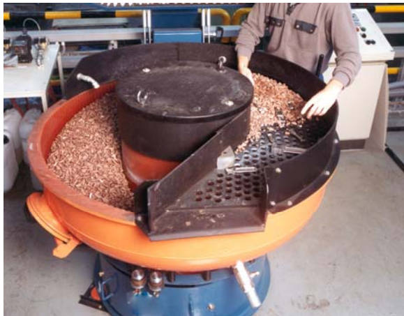
Photo 4; Shows a traditional vibratory bowl. Ideal for processing short stubby parts such as gears, rocker arms, valve springs and bearings.
