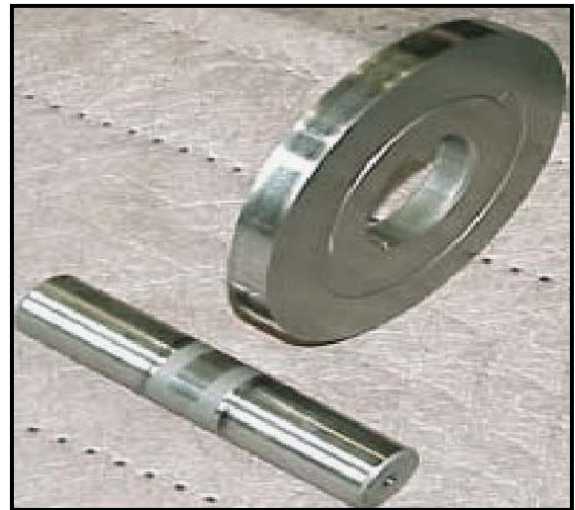
Photo #7; Shows a 1” diameter specimen pin on the lower left and a 5” loading roller on the upper right side of the photograph.
