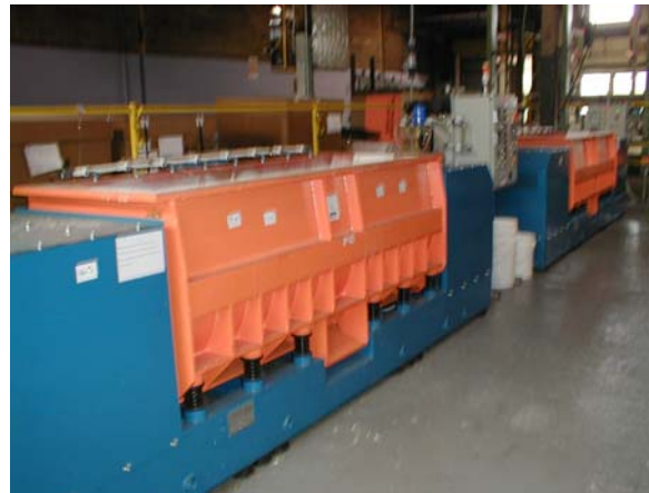
Photo 5; Shows a traditional vibratory tub. Ideal for processing long parts such as splines, camshafts, crankshafts, drive shafts and pinions.
