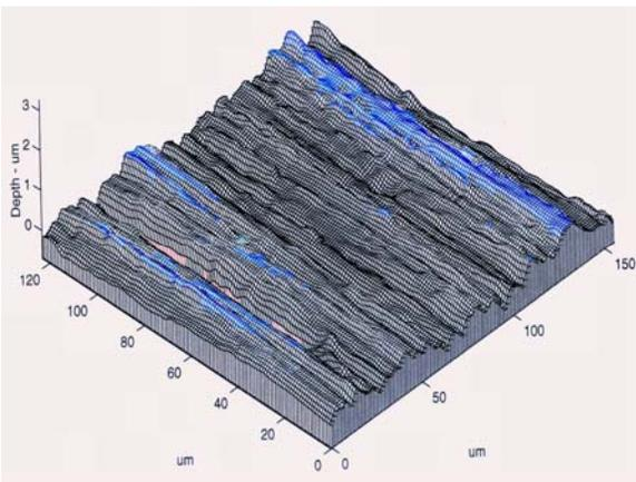
Photo 2; shows a 3-dimensional, 20X magnified view of the surface of a gear tooth that has been ground to a final surface finish of  $R_a = 35 \mu\text{inches}$ . Note the parallel rows of surface asperities corresponding to the directional pattern of the grinding operation.
