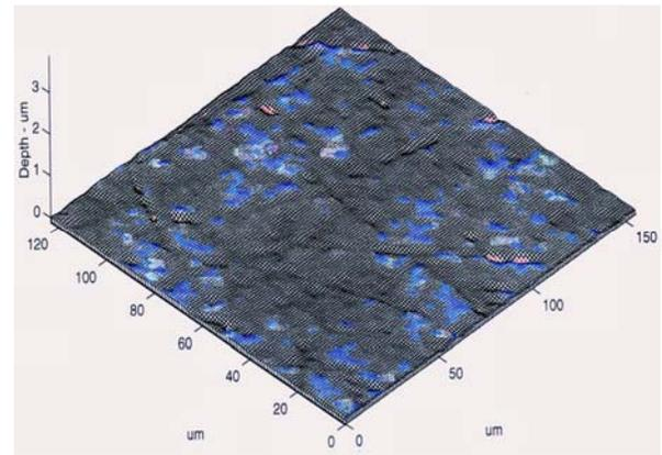
Photo 3; Shows a 3-dimensional, 20X magnified view of an ISF gear tooth. The  $R_a = 1.5 \mu\text{inches}$ . The surface has been produced by chemically accelerated vibratory finishing. Note the elimination of the directional surface asperities (grind lines) when compared to Photo #2.
