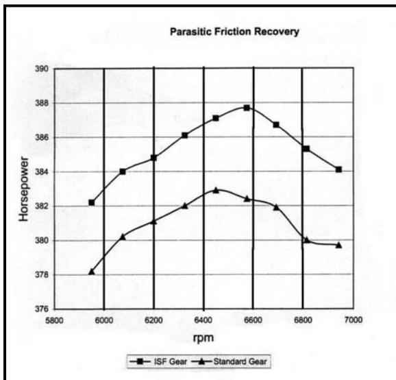
Graph 5; Shows the resultant horsepower graphs at various rpm levels for the tested T 101 transmissions.<sup>10</sup> Note an approximate 1% horsepower recovery with the Isotropic Superfinish transmission.
