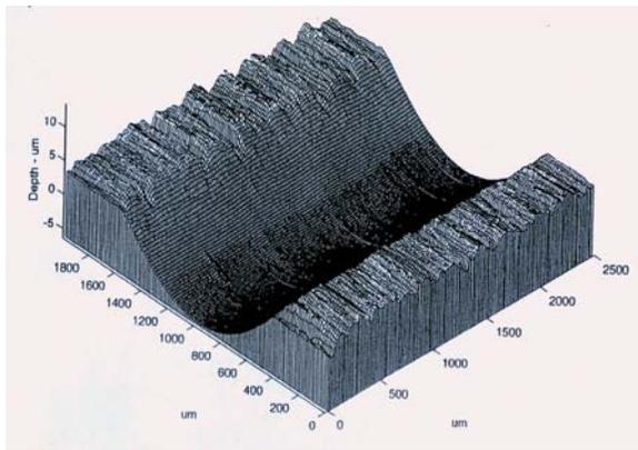
Photo 6; Shows the wear pattern produced in a block-on-ring evaluation<sup>6,7</sup> of a traditionally ground steel block.
