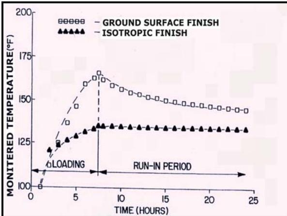
Graph 1; Shows the temperature curves for both the traditional ground specimen and the Isotropic Superfinish (ISF) specimen. Note the temperature spike for the ground surface corresponding to the end of asperity break-in and the complete absence of a spike for the ISF specimen.<sup>2,6,7,9,10,11</sup>
