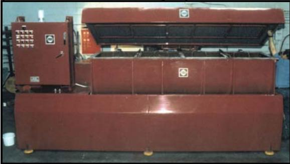
Photo 5; Shows a traditional vibratory tub. Ideal for processing long parts such as splines, camshafts, crankshafts and pinion shafts.
