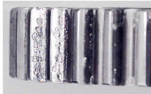
Photo 5; Shows gear tooth spalling caused by surface pit propagation. The gear shown was finished using traditional gear grinding techniques. Asperity peak contact during the gear break-in phase produced micro-pits, that with continued gear operation expanded and eventually coalesced into irregular craters over a significant area of the gear tooth.<sup>6</sup>
