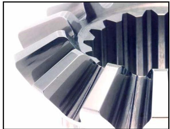
Photo 6; Shows a close-up of the teeth of the bevel gear as shown in Photo 1. The gear was processed using the described chemically accelerated vibratory finishing technique to generate the Isotropic Superfinish. The resultant surface has an  $R_a$  of 1.5  $\mu$ inches. Note when compared to Photo 1, that all grind line asperities have been removed.
