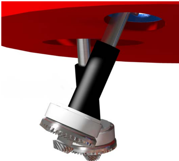
Figure 5: The spindle is attached to the drag finisher with the ring gear and pinion gear held by the magnetic force to the plastic fixture.
