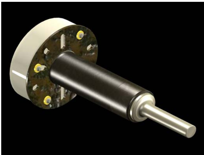
Figure 3: The plastic magnetic fixture shown above and attached to the spindle.
