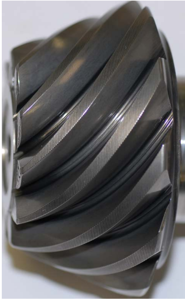
Figure 6: Image of a typical ground OEM pinion after Superfinishing for only 8.0 minutes using drag finishing technology.
