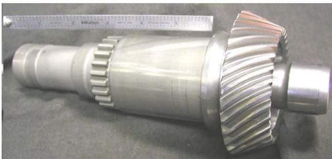
**Fig. 1. 427 ISF processed input pinion.**
