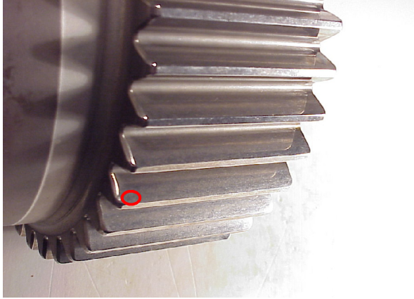
Figure 8. Sun Gear after super-finishing showing that the process eliminated minor FOD. The area circled in red is one of the areas with major FOD that caused this gear to be scrapped.
