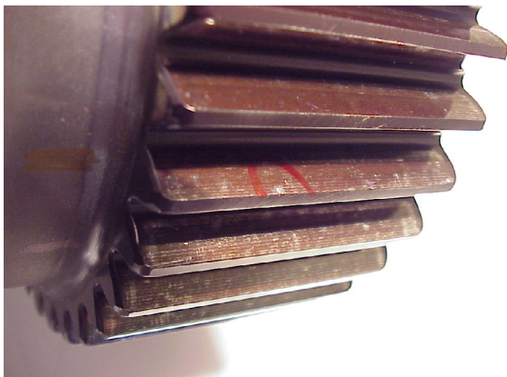
Figure 1. Sun Gear with minor FOD, area circled in red
