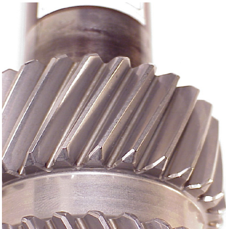
Figure 9. Input Pinion after super-finishing showing that the process eliminated early pitting (gray staining).
